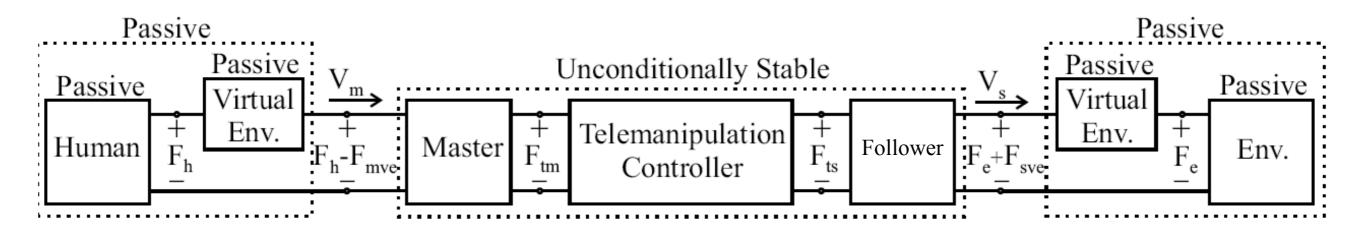
assumptions: system is LTI no sample and hold, no ZOH no time delay or discretization
