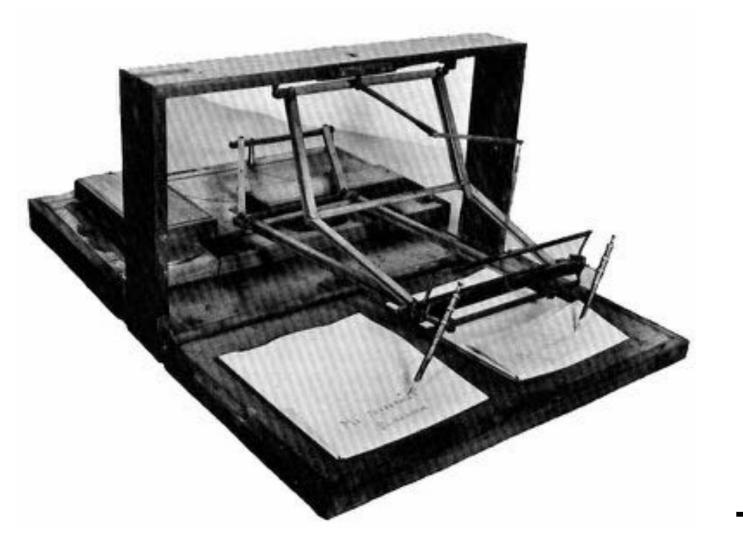
a Polygraph is a mechanical device that produces a copy of a piece of writing simultaneously with the creation of the original, using pens and ink. Famously used by Thomas Jefferson ~1805.
