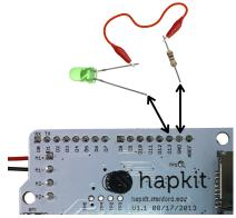
The digital pin 13 outputs 5 V when high. Our LED's specifications are found here:
