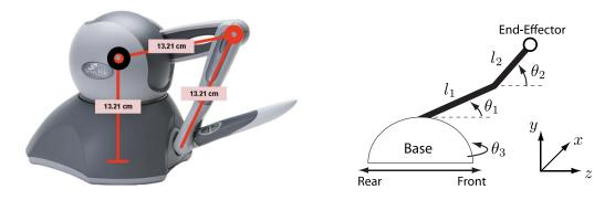
A. Develop a forward kinematic model of the Omni. In other words, compute the x, y, and z positions of the end effector as functions of  $\theta_1$ ,  $\theta_2$ , and  $\theta_3$ . Use the link lengths given in the figure above. The center of the world frame (0, 0, 0) is at the center of rotation of link  $l_1$ . Show your derivation of the kinematics in your submitted solution.
