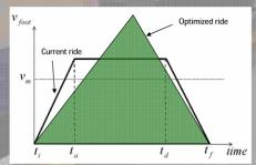
Since the subway has a very well-known route and timing, the acceleration and braking can be optimized. When running at normal time, a computer system will accelerate at maximum efficiency until exactly when regenerative braking at maximum efficiency will stop the subway at the station without coasting.
