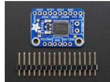
ardumotor shield ( https://www.sparkfun.com/products/9815 ) and Adafruit TB6612 1.2A DC/Stepper Motor Driver Breakout Board
