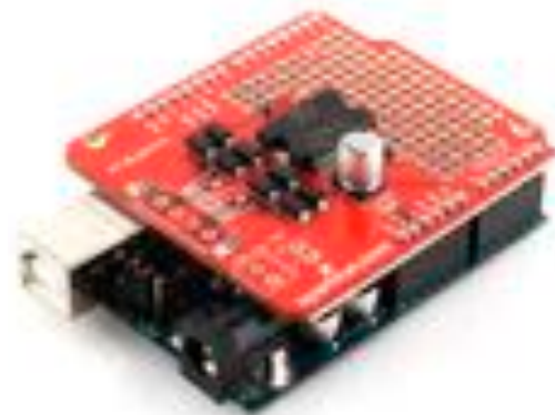
ardumotor shield ( https://www.sparkfun.com/products/9815 ) and Adafruit TB6612 1.2A DC/Stepper Motor Driver Breakout Board
