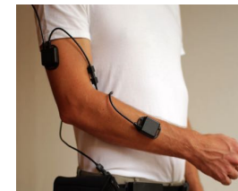
inertial: wearable IMU, MotionNode
