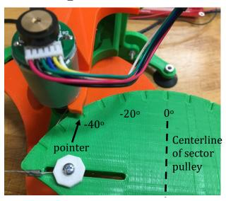
Compile and download this program to your board when the Haplink is in this correct starting configuration, and then check the Serial Monitor in the Arduino environment to be sure that the measurements and outputs make sense.
