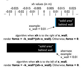
3. Now write code to implement this algorithm in your haplink\_virtual\_environments.cpp file, in the function hapkitRenderVirtualWall. You can copy your virtual spring code as a starting point, and also consider the "if" statement from last week's force output lab.
