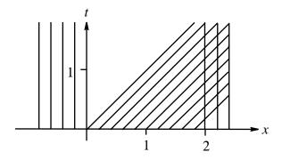
We put in a rarefaction wave in the open wedge and introduce a shock curve where the projected characteristics cross. The rarefaction wave is given by  $G(x/t) = (f')^{-1}(x/t) = \sqrt{x/t}$ . The shock curve  $x = \xi_1(t)$  must satisfy the R-H jump condition,
