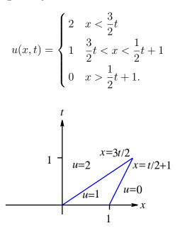
However, at t = 1, the two shock curves intersect. Therefore, the above solution is only valid for  $0 \le t \le 1$ . Consequently, we need to define a new shock curve  $x = \xi_3(t)$
