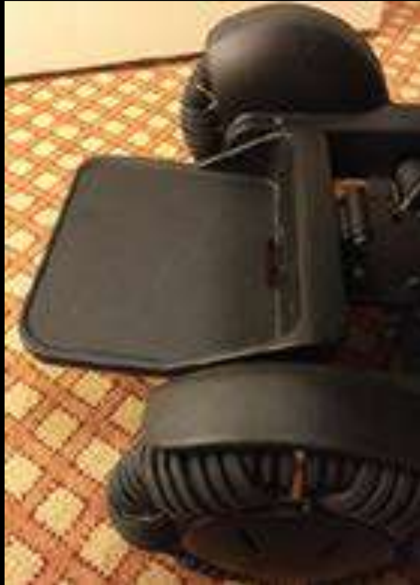
Foot plate comes up when not in use or for smaller storage needs, I put it up in my van.
