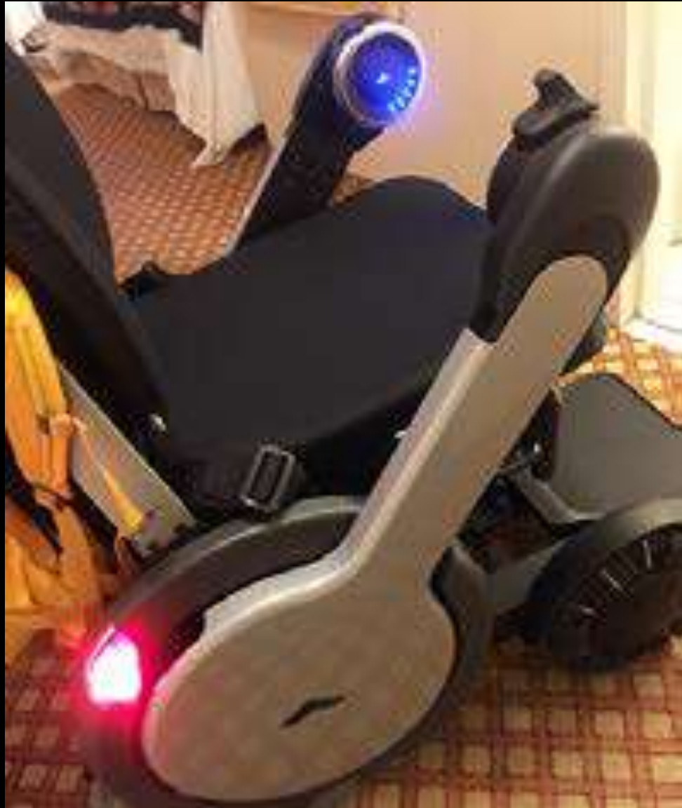
Rear red lights on both sides when turned on. Left front control, blue lights - five when fully charged, with more use less lights lit
