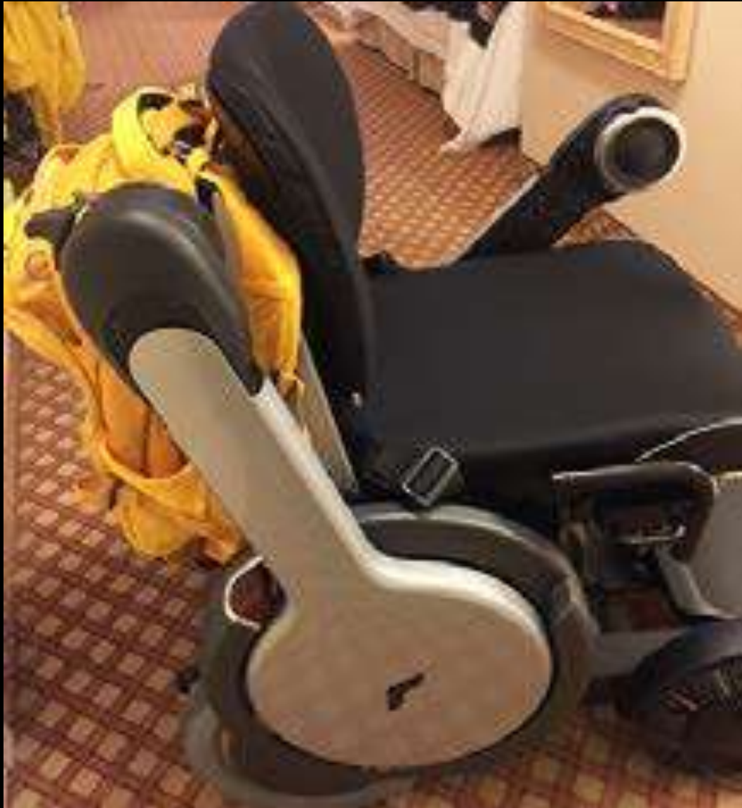
Both arms swing up for easy access. This shows one arm up
