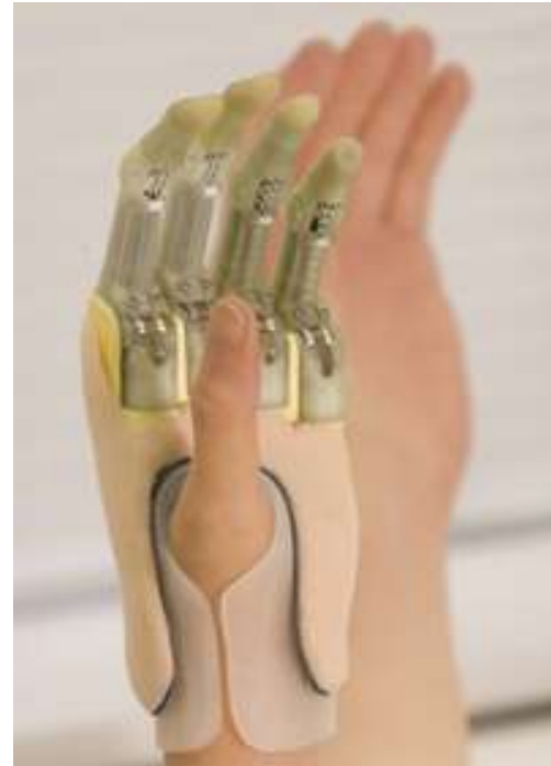
ProDigits – motor-powered prosthetic for those with missing fingers
