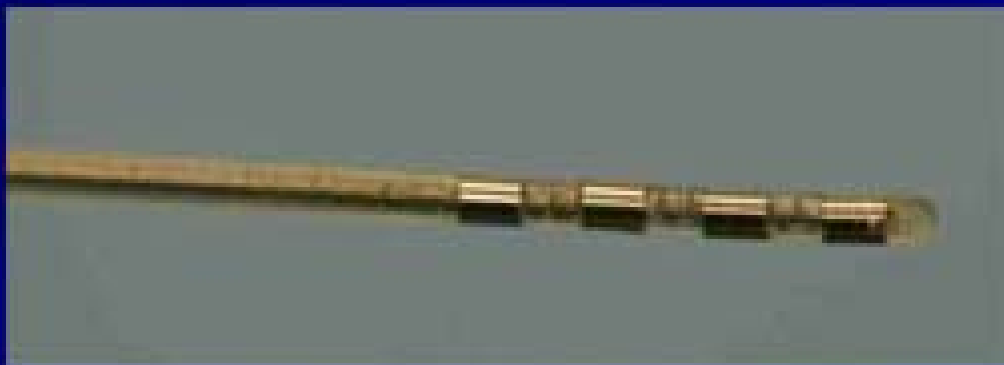
Fig. 1 Scanning electron micrograph of the surface and tip of the control Medtronic 3387 electrode, showing the four potentially active electrical contacts. Bar = 2 mm.
