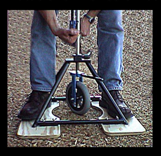
Objective surface measurement device
