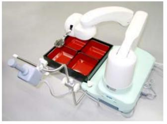
• The device can be tailored for different degrees of disability. The robot is designed for safety: the manipulator, tipped with a spoon and fork, is designed so as not to hurt the user, and its position is set at the beginning of each meal.
