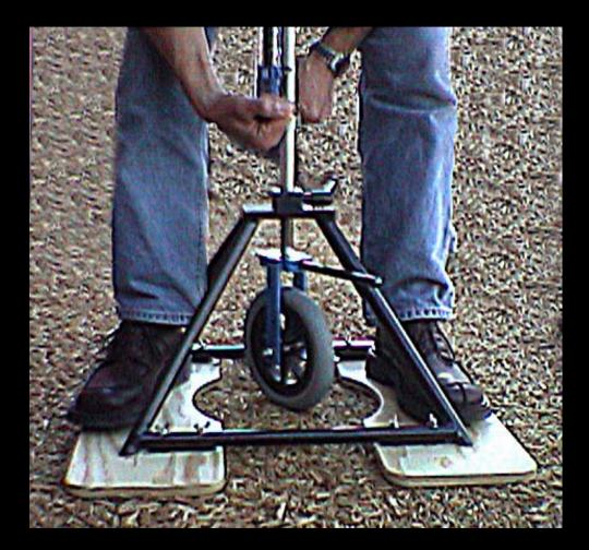
**Objective surface** measurement device **Draft Standard for** firmness with stability measurement under development Available from **Beneficial Designs**
