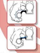
Because the rubber is flexible, the pushrim can compress to allow your wheelchair to squeeze through narrow doorways.
