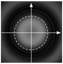
12 turn spiral, 4.5 ms, constant slew rate 1 cm resolution (kmax = +/- 0.5 cycles/cm) SBW = 4 WIndowed jinc RF 220 Hz is one cycle over pulse length
