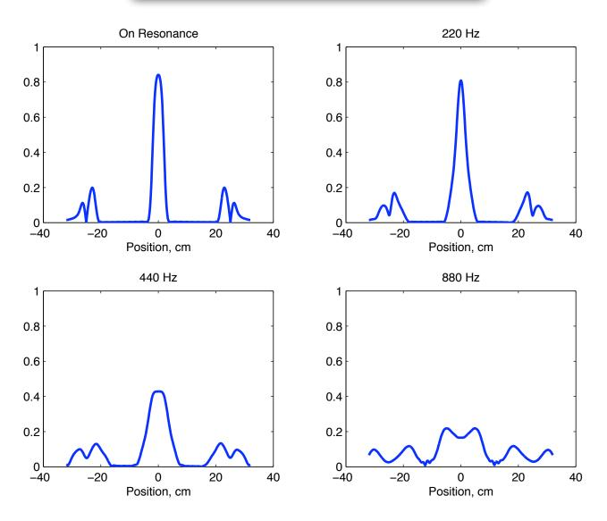
12 turn spiral, 4.5 ms, constant slew rate 1 cm resolution (kmax = +/- 0.5 cycles/cm) SBW = 4 WIndowed jinc RF 220 Hz is one cycle over pulse length
