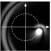
12 turn spiral, 4.5 ms, constant slew rate 1 cm resolution (kmax = +/- 0.5 cycles/cm) SBW = 4 WIndowed jinc RF Modulated to +10 cm along x
