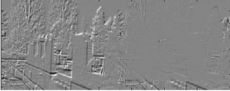
Figure 5: Sample error frame from the Foreman QCIF sequence. Hash-aided motion estimation provides a more accurate estimate of the current frame than that obtained by just using the previous frame as side information. This result is obtained by transmitting a 16 bit hash applied to each 16 \times 16 pixel block of the video frame, resulting in a hash bit-rate of about 0.12 bits per pixel. Note that if a blocks hash is the same as that of its co-located block in the previous frame, then it is not transmitted. Instead, a single bit indicating “No hash necessary” is transmitted.
