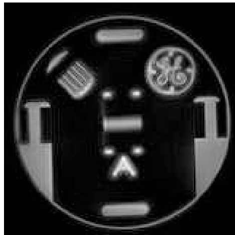
Figure 1: Simple reconstruction of the first data set. While much of the image is in focus, note the blurring around the resolution comb, and the GE logo.
