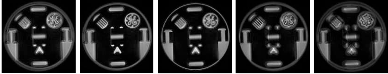
Figure 3: Reconstructions at -128 Hz, -64 Hz, 0 Hz, 64 Hz, and 128 Hz. Note that the structures in the center of the phantom look best at -64 Hz, while the edges look better at 0 Hz, or even 64 Hz.
