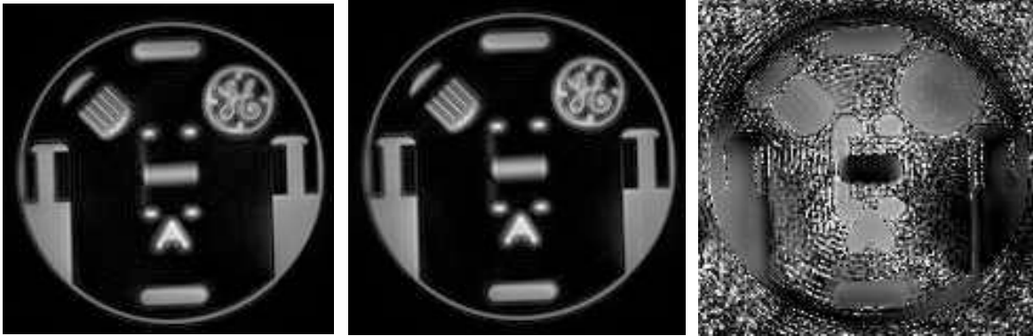
Figure 2: The two data sets look very similar. The first is at at TE of 2.5 ms, and the second at 7.1 ms. The field map shows significant variations in frequency, which correlate well with the off-resonance blurring.
