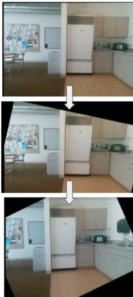
Fig. 6. Result of our Video Stabilization Implementation when moving the phone's camera from right to left and rotating it at a 45° angle. This is from our revised method shown in figure 5.
