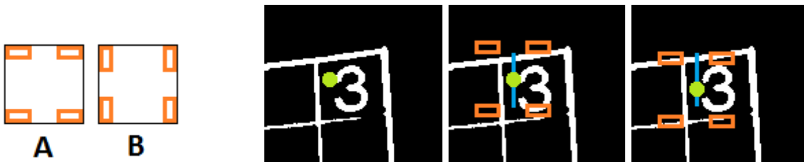
Figure 5. Left: the two structuring elements used. Right: refining a cell center's vertical position using SE A
