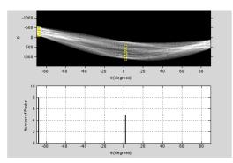
Fig. 2. Hough orientation histogram and peaks
