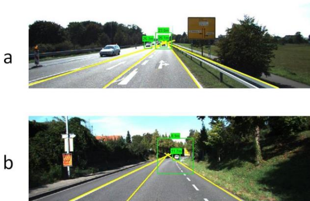
Fig 12. Two screenshots of our algorithm running poorly on dataset from KITTI for lane detection.
