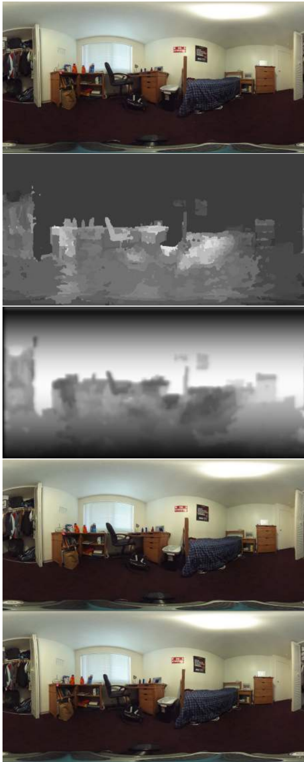
Figure 6: Images from top to bottom: original lower image, segmented disparity map, depth map, left view, and right view.
