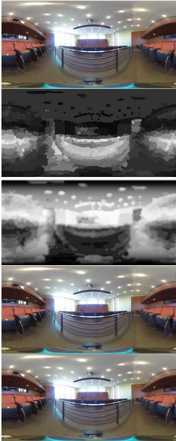
Figure 8: Images from top to bottom: original lower image, segmented disparity map, depth map, left view, and right view.
