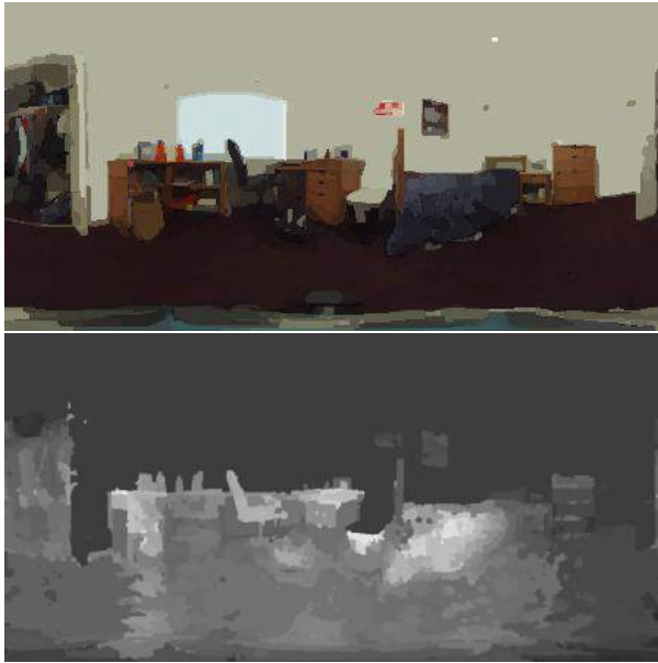
Figure 5: The top image is the room segmented by color. The bottom image is the resulting disparity map after averaging the segmented sections.
