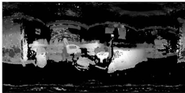
Figure 3: The disparity map with the noisy regions zeroed out. The disparity map now appears a lot cleaner
