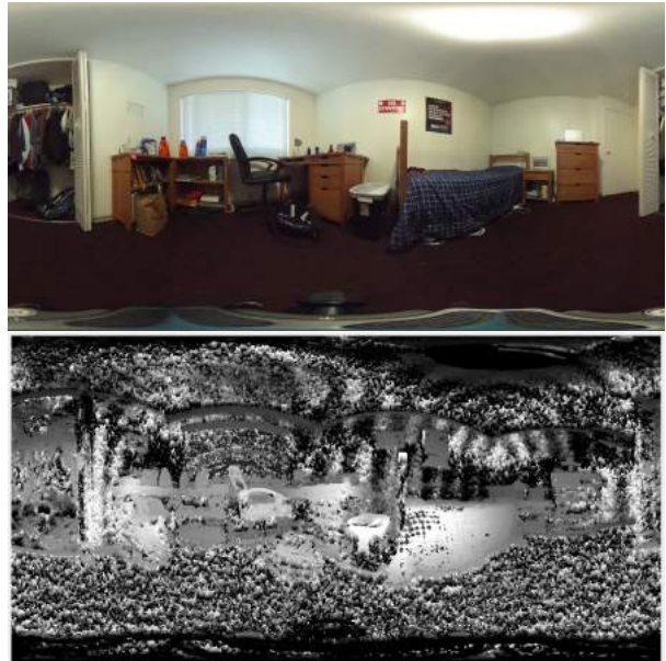
Figure 2: The top image is the lower image taken by the Ricoh Theta. The bottom image is the initial disparity estimation. Brighter pixels correspond to greater disparity and therefore closer image
