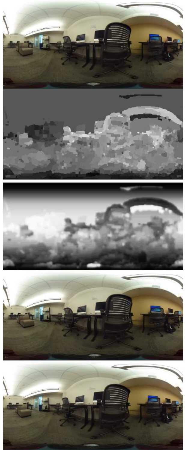
Figure 7: Images from top to bottom: original upper image, segmented disparity map, depth map, left view, and right view.
