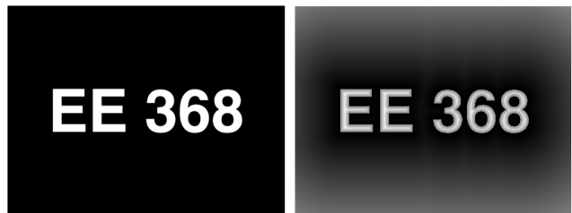
Figure 2. Before and after morphological image processing
