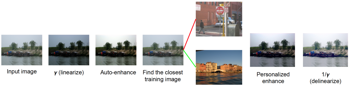
Fig. 4: Image Processing Pipeline to Personally Enhance Newly Added Images
