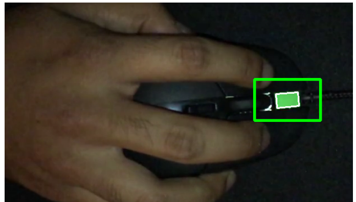
Fig. 5. Calibration - The initial calibration step determines the location of the tracker using the HSV channel and a bounding box around the tracker which the subsequent frame will use as the region of interest.
