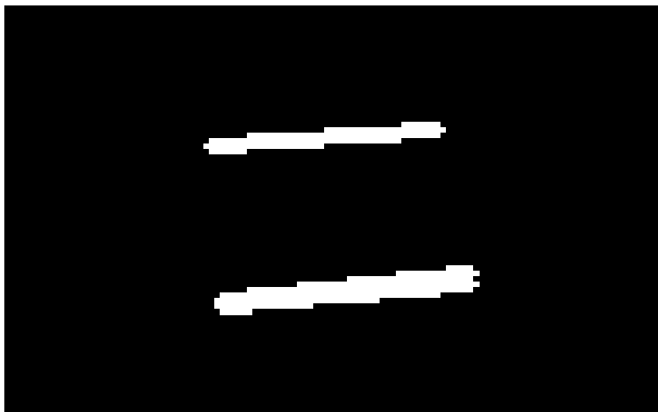
Fig. 9. Probabilistic Hough Transform - Calculates the tracker rotation, used to normalize the tracker and compute the offset from the centroid to the mouse sensor, 4.5 \times [\text{long side of the tracker}] .
