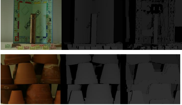
Fig. 3. Modes of failure. Left: original, middle: ground truth, right: graph cut results. The combination of ambiguous geometry, untextured surfaces, and occlusion leads to large errors. The image above features untextured surfaces on the wall and the board, as well as an occluding object in the middle and many occlusions in the foreground. The image below features ambiguous features whose depth cannot necessarily be resolved by stereo correspondences.
