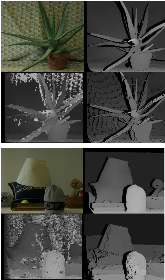
Fig. 2. Disparity algorithm results. Upper left: source image, upper right: ground truth, lower left: NCC algorithm, lower right: graph cut algorithm
