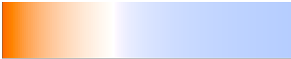
Figure 3 Temperature to RGB value from 1500 K to 5000 K [6]. High temperatures seem blue and low temperatures are orange-red.
