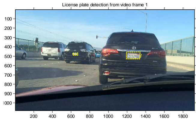
Fig. 7. Detected license plate highlighted in original image
