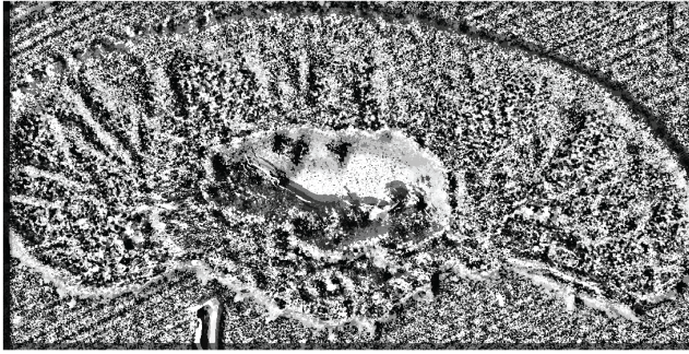
Fig. 2. The result of finding Local Binary Patterns (LBP) in an EM image. Grayscale value correspond to different LBPs, i.e. different arrangements of relative grayscale intensity around each pixel.
