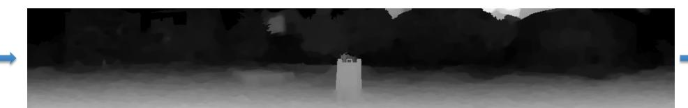
Disparity map: We observe uniform gradient of disparity along the ground plane, in the bottom half of the image.
