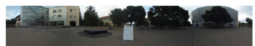
**Original lower image**: Equirectangular projection (altitude -30° to 30° and azimuth 0° to 360°) with good mix of obstacles at various ranges.
