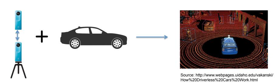
The objective is to detect obstacles in the surroundings using stereo vision from 360° spherical images captured from vertically displaced cameras.
