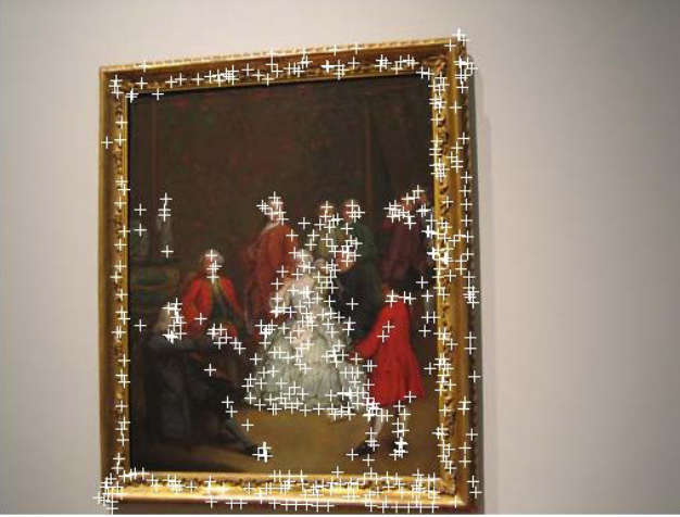
Figure 3: Stable keypoints after removing the edge elements
