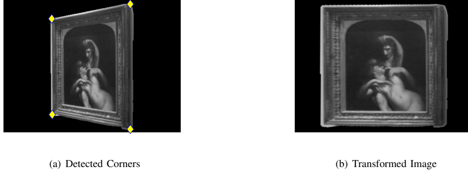
Fig. 3. (a) Corners detected using the four quadrant method on masked image. (b) Final output image from pre-processing stage.
