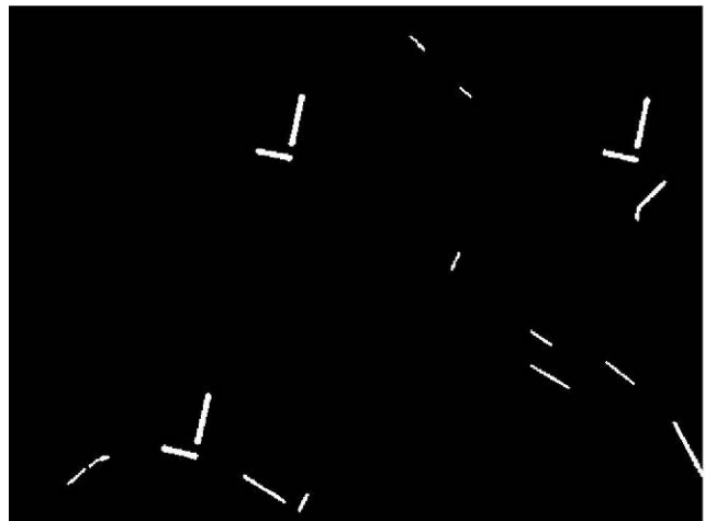
Fig. 4. When locating regions corresponding to guide bars, many regions are eliminated because they are too small, or do not meet the typical eccentricity range of a guide bar. After this elimination, the relational geometric properties of two regions are evaluated to identify which pairs represent code marker guide bars.
