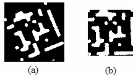
Fig. 8. (a) Detected portion as it appears in the binary image; (b) Portion rotated to square and trimmed of excess area.
