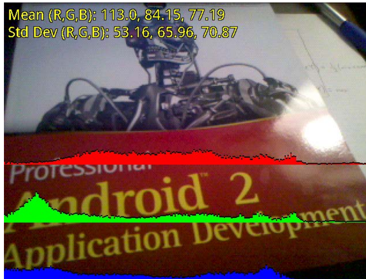
Figure 2. “Viewfinder EE368” program running on an Android phone. Demo video: http://ee368.stanford.edu/Android
