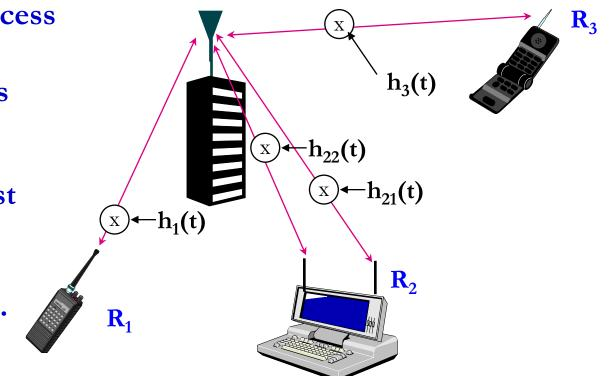
**Uplink and Downlink typically duplexed in time or frequency Full-duplex radios are being considered for 5G systems**
