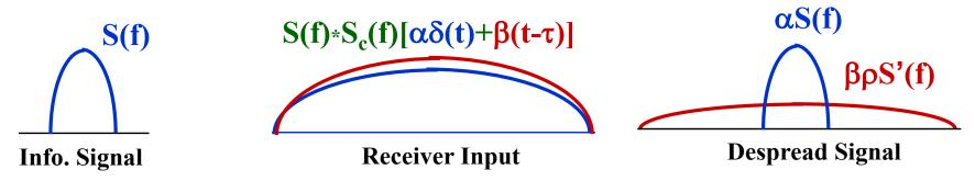
Can coherently combine all multipath components via a RAKE receiver
