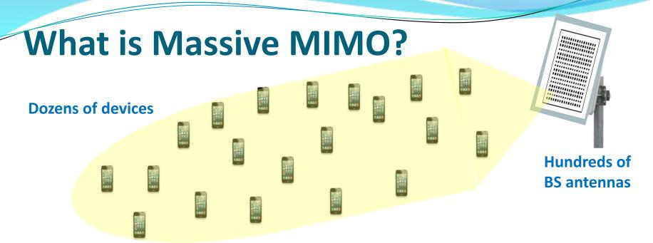
A very large antenna array at each base station
