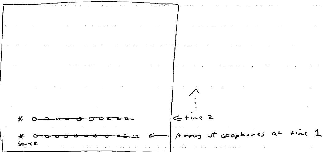
where the array of receivers and the source are moved up the area to be surveyed. Here a linear section would be traced out upward under the assumption that the depth of each layer is constant under the array from left to right.
