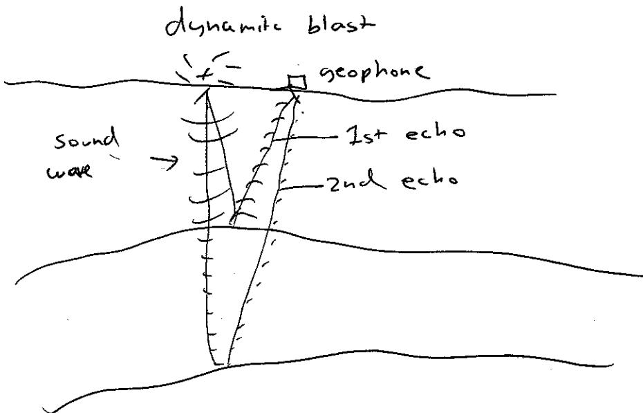
A large sound wave propagates from the dynamite, to the layer, and back to the geophone. If there are multiple layers each has an echo associated with it. The first echo comes from the top layer, then each successively deeper layer.
