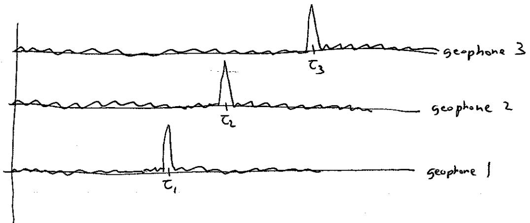
where the depth  $d$  is related to each geophone spaced  $s_i$  and results in an echo at  $\tau_i$ :
