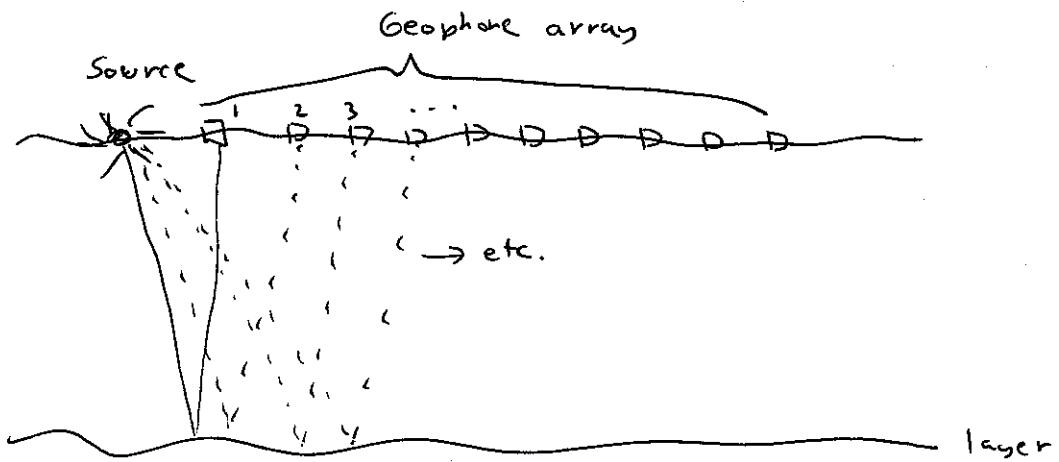
If the layer is locally flat, the time delay of the echo depends only on the separation of the source and detector, as well as the depth. Traces might look like
