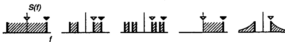
Figure 7-8 Some band arrangements meeting the condition S(f) = 0 wherever |f| > f_{\max} or |f| < f_{\min} and one (on the right) that does not.
