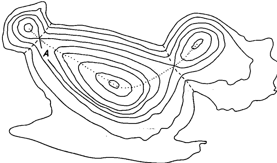
Figure 2-15 An island with three unequal tops and two saddles at the same height. Four watersheds and four watercourses are indicated. There are no bottoms above sea level.
