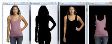
Solution: Increasing Skin Threshold removes pixels that are less likely to represent skin.
