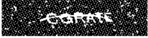
Fig. 3. k -means with radius and pixel intensity. Non-black pixels are made white.
