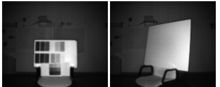
Figure 3: Intensity images provided by the depth sensor. To gather data for our noise model, we collected data of a Macbeth check at different distances and of a board at different orientations and distances.
