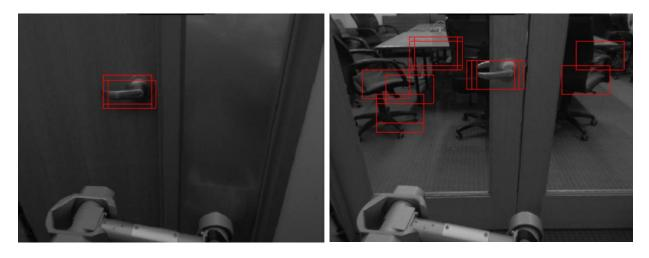
Figure 2 – Sliding Window results for (a) opaque and (b) glass doors
