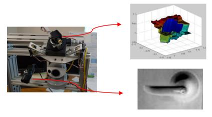
Figure 1 – Visible light laser with a camera is used to obtain the image of a door handle and the corresponding 3D point cloud view. Image pixel values and corresponding X-Y-Z coordinates are used as feature vectors.
