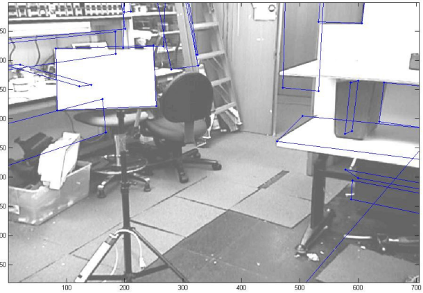
Figure 6: Calibration based on 4 points – TL, BL, BR of easel, BL of desk. Heuristic = 455.9.
