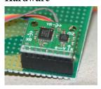
To increase the amount of information available to the gesture recognizer, we've used a five degree-of-freedom inertia measurement unit (IMU) combination board. The board includes the 3-axis Analog Devices ADXL330 accelerometer chip providing accelerations in X, Y, and Z axes and the dual-axis Invensense IDG300 gyroscope chip providing roll and pitch.
