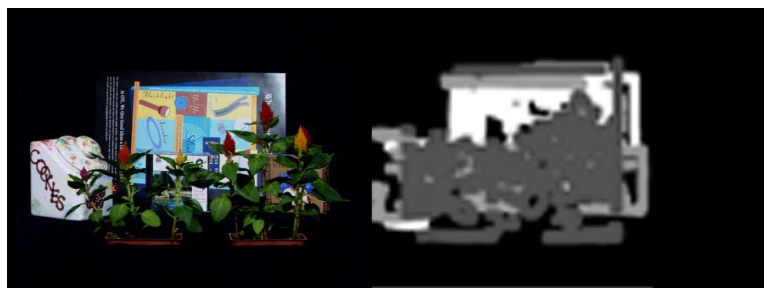
Figure 4: Depthmap created from real data using Stanford Camera Array. Left: original image from one camera. Right: computed depthmap. Significant improvement over images with no texture is made in images such as this with lots of texture variation.
