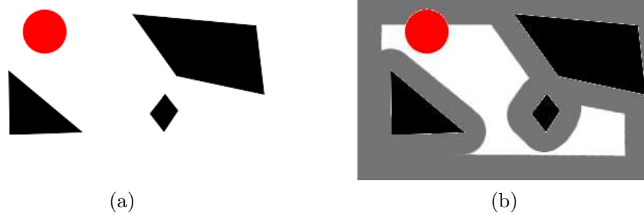
Figure 2: (a) An example workspace with the circular robot shown in red. (b) The resulting configuration space, where the white areas are the free space. Coordinates are defined with respect to the center of the robot.
